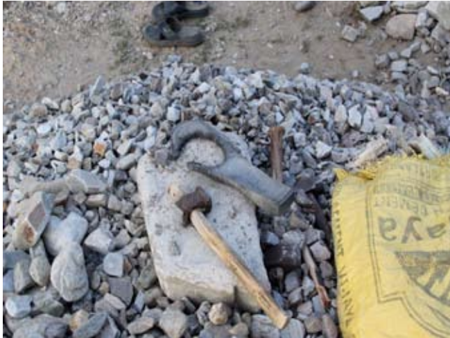
Tools for crushing stones: hammer, stone holder, and bag to sit on.
